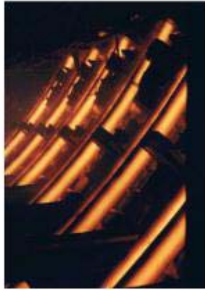
Figure 7 - Curved Section of Multi-Strand Beam Blank Caster prior to Unbending
