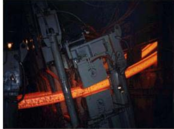
Figure 8 - Straightener Withdrawal Units for Strand Unbending
